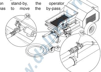
lever (20)recycling position (vertical). At the next start up the before mentioned lever has to be placed in pumping position (horizontal).
