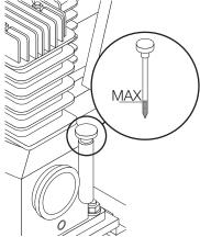
In a building site the compressor seldom works in perfect horizontal position as suggested by Turbosol, therefore in order to obtain a correct lubri-
