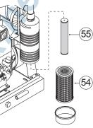
Hit, gently various times the air filter element 1° (54) on an hard surface in order to remove the dirt. It is not advisable to blow with compressed air the paper element.
