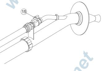
Generally with smaller size deflectors material is sprayed with a wider spray pattern and vice versa.
